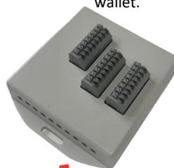
The TQ-SLU (pictured left) shares a lot of components with the TP-SLU but is suitable for machines that use a pulse line to apply credit. The unit is also based upon a Raspberry Pi and secure software developed by Polar Moment.
